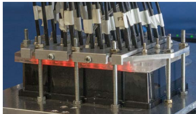
Novel miniature test system ( \mu RAMOS) , enabling determination of respiratory activity in each well of a microtiter plate thus spotting PrimACs.
