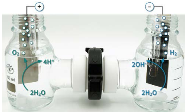
Design of the electrochemically induced separation method: two electrode cages each with cathode (left) and anode (right), agitators and intermediate membrane.
