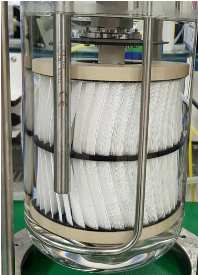
Module for bubble-free membrane gassing integrated into a bioreactor.
