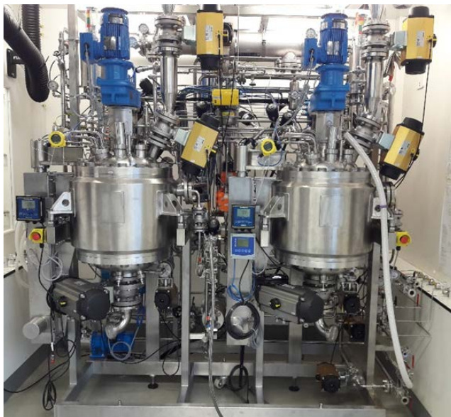
Fractionation reactors for realizing the OrganoCat-process in the pilot biorefinery NGP 2 at RWTH Aachen.
